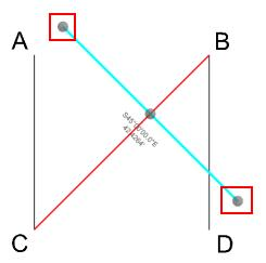
R. Previously there was a snap Civil Rule at end point A because when the initial line segment was created the user snapped to the end of the line. This created a Civil Rule. By using the midpoint drag handle the user has broken the rule. Select UNDO (Ctrl+Z) to undo the move, this will also undo the process of breaking the Civil Rule, it will reestablish the snap rule, indicated by the icon at Point A.
