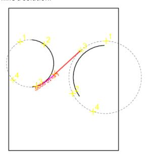
K. Left click to accept the End Offset Value = -2.00. Note that the sign updated to (-) to match the solution shown on the outside of the Arc.
