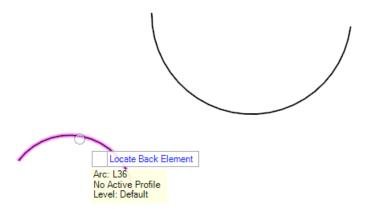
S. Left click to set the offset distance to -2.00, this will put the offset to the outside of the arc.
