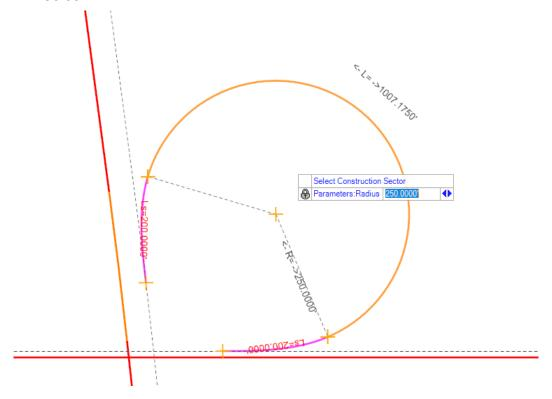
N. No trim option will appear because the loop ties to offsets of the reference element. This completes the placement of the loop centerline.
