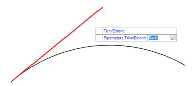
P. Note that the arc was trimmed to match the line segment. The program will trim or extend the arc in the appropriate direction to match the tangent direction of the line segment.
