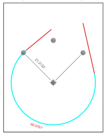
R. The radius can be adjusted by using the drag handles or the text manipulator. Note that the length 90.0761' is shown in red, this indicates that the length Text Manipulator cannot be revised, in this case that is because it would change the center location and there are no rules to tell the program how to change the center location.
