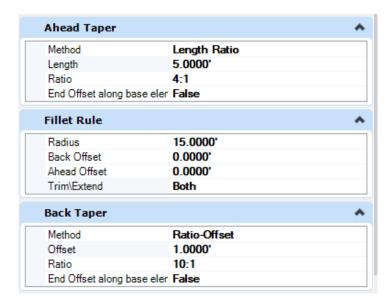
M. This will produce an Arc with two linear tapers and will reestablish the trim of the two base elements to match the tapers.
