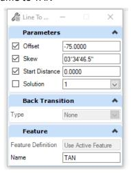
V. Left click to select the L line as the To Element. Use the Pick Complex Element Option because the tie point of the Collector Distributor is not yet known. Note the heads up prompt displays the unselected option.
