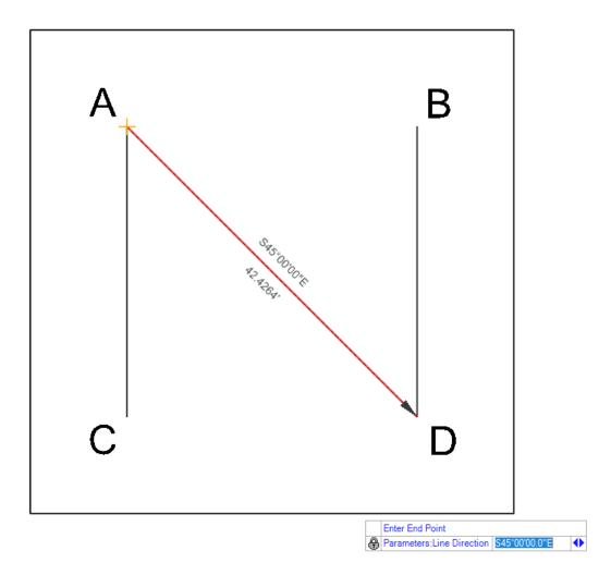
P. The screen should match the picture above with the line starting at Point A and ending at Point D. The length and bearing are shown on the line. This line has not yet been placed in the file this is a tentative location.
