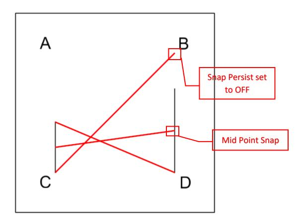
Q. Because the Snap Persist setting was inactive when placing the line from C to D that element did not update when the change was made to line from B to D. Note that the horizontal line again updated to maintain the Mid Point Snap based on the new line length.
