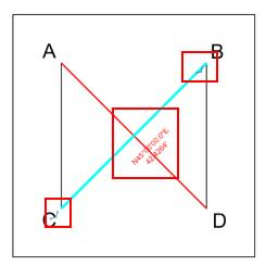
W. Remember that the drag handle can break the civil rule. With the line selected move the cursor close to the end at Point C. The gray circle will appear with the two gray arrows indicating the drag handles.
