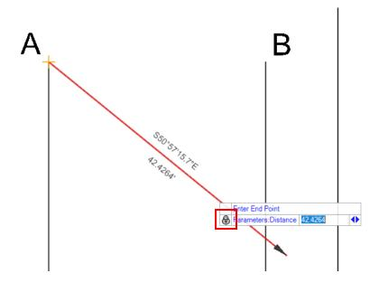
If focus has been lost from the design window click on the Border to bring it back and activate the entry field. Do Not click in the drawing field or the end point of the line will be selected.
