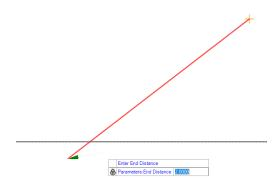
A negative (-) Distance will place the end point on the same side of the From Element as the initial point selection. In this example above the line. The distance will be measured along the skew from the From Element. A small distance would put the point between the From Element and the initial point and a larger distance would place the point further away from the From Element than the initial Point.
