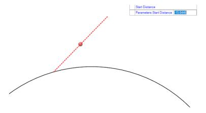
K. By left clicking in the correct location initially the user will be prompted for the start distance. This is the distance from the To Element as measured along the Proposed line where the program will place the starting point of the line. At the heads up prompt enter 2' and press the <ENTER> key.
