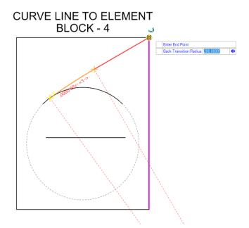
I. Note that even though the dialog box was filled out with the appropriate design data the user still has to left click through each option in the heads up display to accept the previously entered data for radius and transition.
