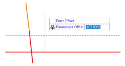
O. Snap to the intersection of L and Y8. The Persist Snap is set to OFF so this will not create a snap rule.
