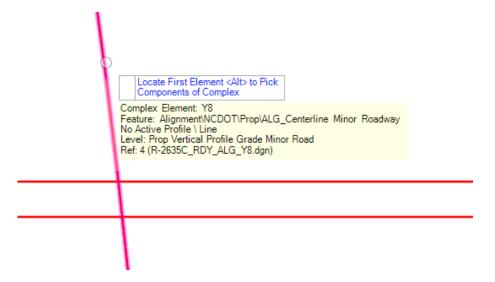
J. Left click to accept the offset of 47.50'. Note that the dashed line representing the offset follows the Y8 alignment not the extension of the tangent on Y8.
