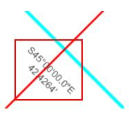
G. One way to edit the civil geometry is by editing the length and/or bearing shown in the Text Manipulators. With the line selected select the green length text at the midpoint of the line. A data entry field will appear with the current line length shown.
