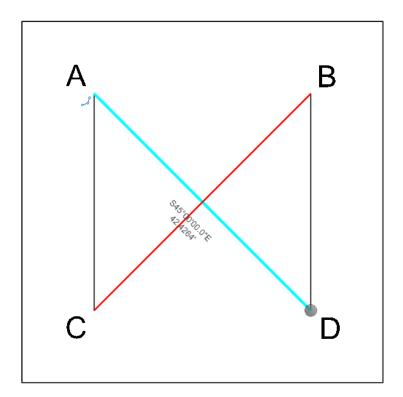
C. Note the symbol next to the A, this indicates that a Snap Civil Rule was created for this point when the line segment was created.
