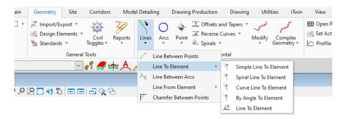
This group contains tools that will allow the user to draw a line segment that will be based on another element. These tools will be used when construction Horizontal Alignments, especially for construction Y Lines, Intersections, Ramps and Loops. Additionally this group of tool sill be used when constructing other civil geometry features that will be covered in other Modules.
