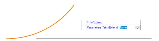
M. The Trim/Extend option will display none because that was the selection made in the dialog box. Left Click to accept the solution and complete the tool.
