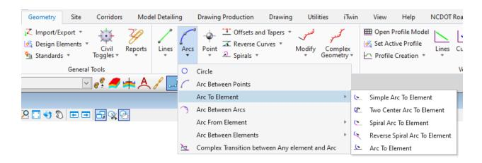
This group contains tools that will allow the user to draw an arc that will be based on another element. This group of tools will function on the same concepts outlined in the Line To Element tool group, the user will specify a point in space where the Arc will begin and then the program will draw that arc To the specified element.
