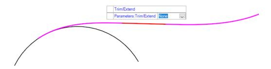
L. This will complete the tool, place the element and trim the From Element to match the transition spiral.
