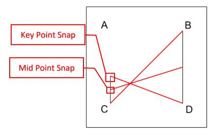
O. Because the Persist Snap Rule was Active when the line from A to D and the horizontal line were placed those two lines have updated to maintain the rule. The Line from A to D has maintained the Key Point Snap at the end of the reference line and the horizontal line has adjusted to maintain a snap at the Mid Point of the shortened line.
