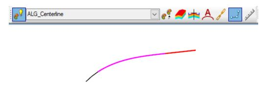
K. Left Clicking on the element will display the drag handles and the text manipulator that can be edited. This will work in a similar way to the Simple Line to Element tool. In this case it is only the ned point location and the length of the spiral.
