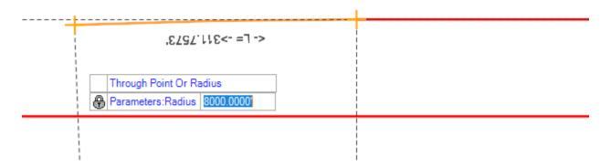
OO. Left click to dynamically accept am Arc Length. This length can be any value. During the placement of the reversing curve the trim option can be set to back and the curves will adjust to tie at the tangent point.
