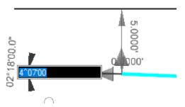
R. This is another example of how geometry rules and design intent could be used to modify a horizontal alignment. If a ramp alignment was built off of this as the initial tangent a change to the skew angle would result in modifications to all the curves, spiral and tangents to maintain the design intent of the ramp alignment.
