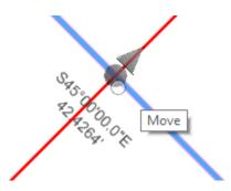
T. Move the cursor up and to the right towards Point B. This drag handle resets the midpoint of the line segment. Note that this drag handle did not break the snap Civil Rule at Point A. So the beginning point of the line stayed in the same location, the end point moved based on the new midpoint.
