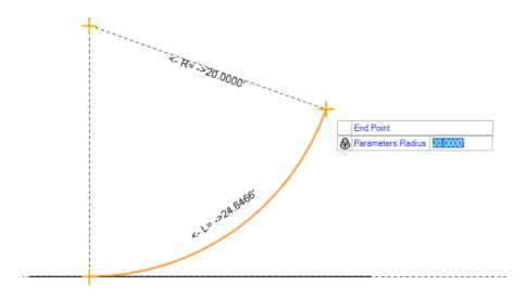
H. To move the curve to the opposite of the line, from the Top to the Bottom just move the cursor from the top of the line to the bottom of the line.
