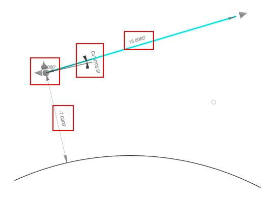
N. This line now starts at a point 7.0' to the left of the From Element at a skew of 3°30'00" and has a total length of 15.00'
