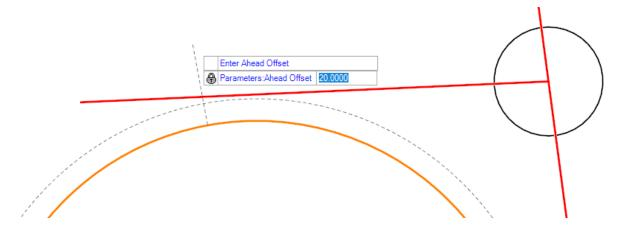
V. Position the cursor in a location that shows the desired solution and left click to accept the radius of 600.00'
