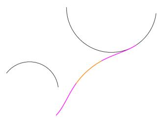
Z. Use the Element Selection tool to highlight the element and note that the spiral ties 2.00' offset from the project of the Back Arc. There are reversing spiral transistions at each end and an arc with a radius of 20.00' in the middle.
