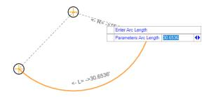
K. Left click to set the end point and complete the arc placement.
