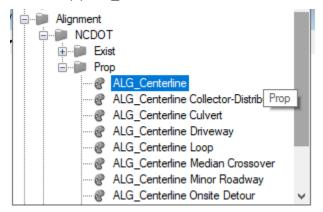
It is important to select the Feature Definition that corresponds to the type of roadway centerline being designed. The featured definition will control the display properties of the centerline annotation and each type of alignment has different standards.
