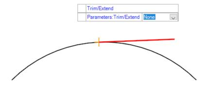
H. This will set the end of the line and bring up the Trim/Extend option. Use the Down Arrow to change the option to Back.
