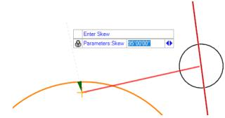
By placing the cursor below the line the skew angle is located below the line.
