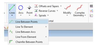
F. Draw a line from Point A to Point D snapping to the ends of the black lines.
