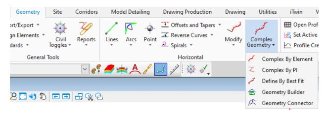
R. The only task left to accomplish is to Station the Complex Element. The Loop Alignment starts at Station 5+00.00 at Y8. Select the **Start Station** tool.
