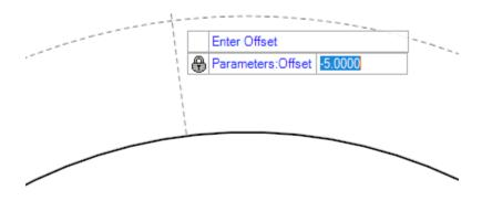
G. Left click to select the Start Point, this is not the start point of the line, this is point where the tool starts the construction of the line. The line will pass through this point. This point will be located at the specified offset from the From Element.
