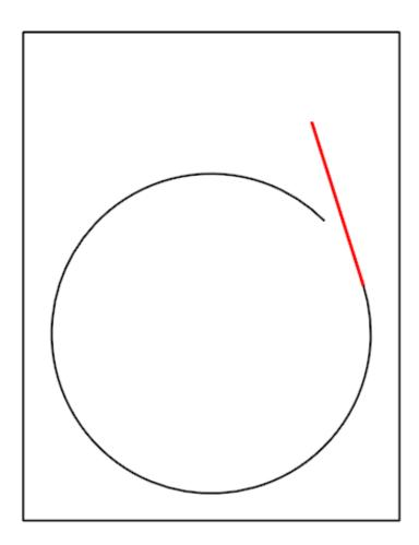
Because the Back option was selected for the Trim/Extend Option the program created a solution that extended the base Arc element around to the Line element.
