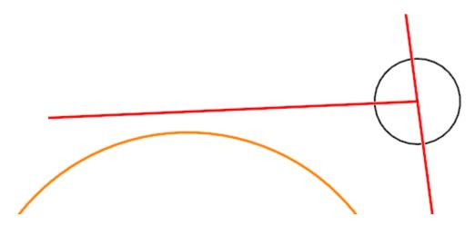
P. The next step is to construct a curve with a radius of 600.00' that is 20.00' offset from the Loop centerline. Start the **Arc Between Elements** tool.
