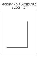
B. Set the Feature Definition to ALG\_Centerline and using the **Arc Between Elements** tool construct a simple Arc with a radius of 10.00' between the two elements and trim both.
