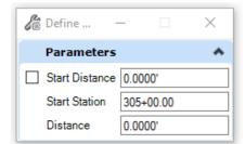
beginning of the element when the start station command is started this value will change to a station value and the distance box will show the distance from the beginning of the alignment. This is useful if a Start Distance other than 0.00' is determined graphically.
