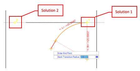
P. The user can switch between these solutions by using the <a href="ALT">ALT</a> key. This is common across all the tools when there are multiple possible solutions. Also note that the program will use the extension of the To Element to determine a solution.
