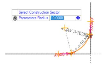
H. Left click to accept the Trim option of Both. This will complete the tool and place th Spiral Curve Spiral combination. This also trims the reference elements to the spiral transitions.
