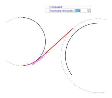
O. The ends the tool and completes the process. Note the back element was trimmed to meet the spiral transition.
