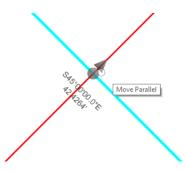
P. Select the arrow to move the line segment parallel. Left click to accept the new line location.
