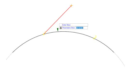
I. Left click again to accept and set the end point. When left clicking this time it is important to select a point in between the initial end point and the To Element. By Left clicking to accept the end point the user is also initializing the Start Distance.
