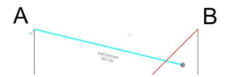
K. The circular drag handle will allow the user to change the length and direction at the same time. When selecting the circular drag handle both individual drag handles will appear.
