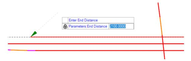
R. That will place the central tangent of the Collector Distributor alignment.
