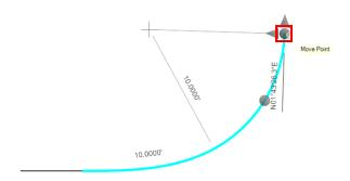
J. Pull the curve to left, note that the spiral will move and the To Element, the line segment, will update to maintain the Back Trim.
