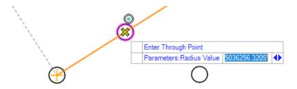
P. Snap to the center of the circle on the right and left click to select and accept the end point. The dynamic display should indicate the radius is 10.00'
