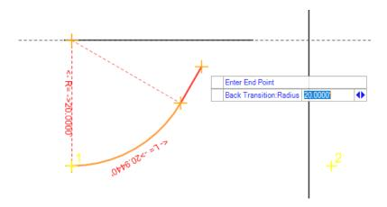
N. Move the cursor far enough away from the line to allow the curve to solve and the dynamic solution will show a curve tangent to the line.
