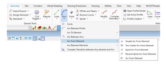
This group contains tools that will allow the user to draw an arc that will be based on another element. This group of tools will function on the same concepts outlined in the Line From Element tool group.
