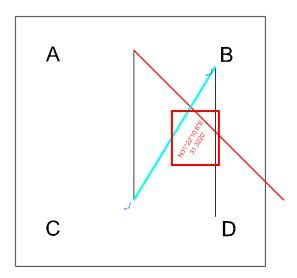
H. The line from Point A to Point D has changed in a different way. The beginning has stayed at Point A, this is where the Snap Constraint was located. The end point that was at Point D has shifted, this is because there was no constraint at that point so the line segment has maintained the original distance and bearing.
