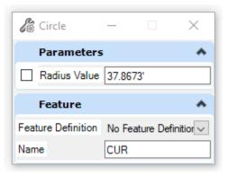
E. The heads up display will prompt for a center point. Snap to the middle of the line and left click to accept the center point.
