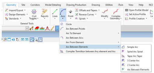
This group contains tools that will allow the user to construct an arc between two previously placed elements. This tool has the ability to optionally apply a back and/or forward transition and/or taper between the elements and the constructed arc. This tool group will be commonly used by the roadway designer.
