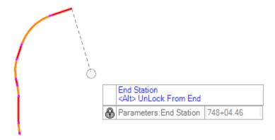
F. Set the interval to 0.00. For a number larger than 0.00', additional points, computed event points, will be added to the report. These reports will be spaced along the alignment at the specified interval and can be used to display information like stations, coordinates or elevations. Left click to accept.
