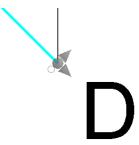
G. The drag handle that is parallel to the line will Trim or Extend the line. By left clicking to pick the arrow the user can change the length of the line.
