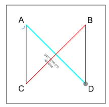
O. Move the cursor near the midpoint of the line to show the move parallel drag handle represented by the arrow.
