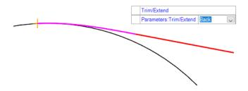
I. This will trim the From element to the end of the spiral transition and complete the tool
