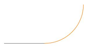
P. When the radius is edited to 10.00' the point on the To Element moves to match the new radius. This is the opposite of the From Element tools.
