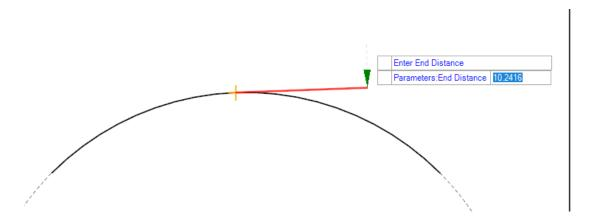
G. Enter the line length to set the end location using either positive number to set the line direction up or to the right. A negative number to set the line direction down or to the left. Or left click to accept the end location. Note that by left clicking the end point will always be a positive solution.
