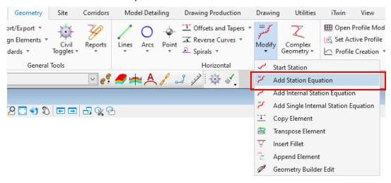
C. At the dialog prompt enter 444+99.34 for the Ahead Station and 445+12.10 for the Back Station. Check the box for back station to lock the value. Note that the ahead station must be preceded by a name, in this case S2 to represent Section 2
